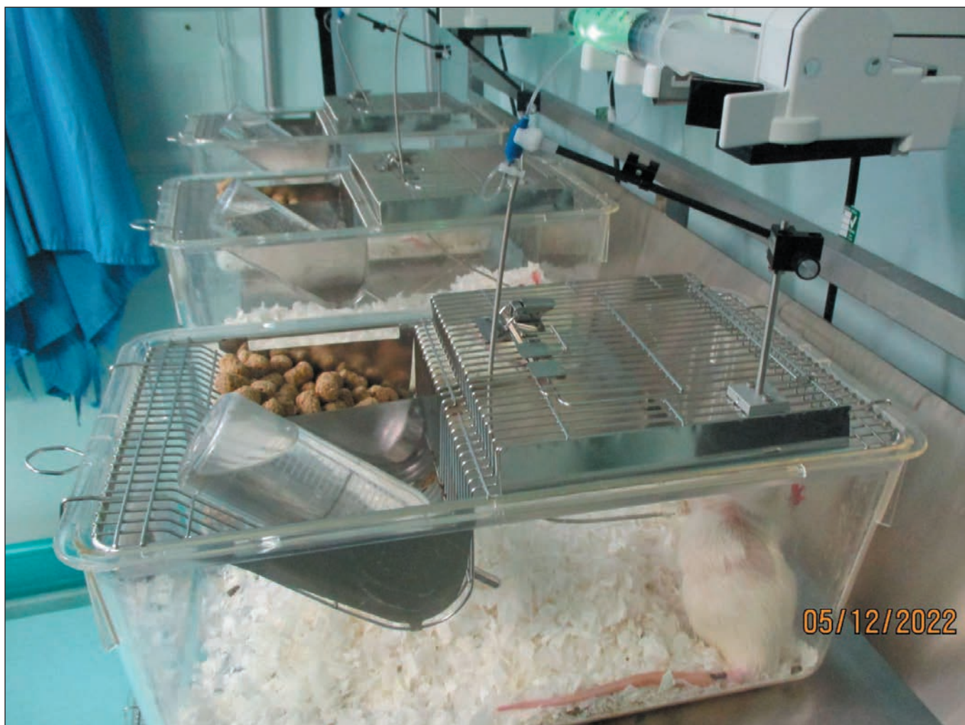
Figure 7. Cage setup with lever arm to support dosing equipment.
